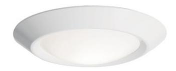
TRIM COLOR N/A BODY FINISH White WATTAGE 14.5W/ DIMMER Dimmable DIMENSIONS 7.38"W x 1.25"H INTEGRATED LED MODULE LAMP 1 x LED/14.5W/120V LED Technical Information LUMINOUS FLUX 1000 lumens LUMENS/WATT 68.97 LAMP COLOR 3000K COLOR RENDERING 90 CRI SPEC # JUN472532
