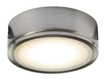
SHADE COLOR Frosted **BODY FINISH** Satin Nickel WATTAGE /<sub>1</sub> 5\\\/ DIMMER Low Voltage Electronic DIMENSIONS 2.75"W x 0.94"H INTEGRATED LED MODULE 1 x LED/4.5W/120V LED LAMP Technical Information LUMINOUS FLUX 200 lumens LUMENS/WATT 44.44 LAMP COLOR 3000K
