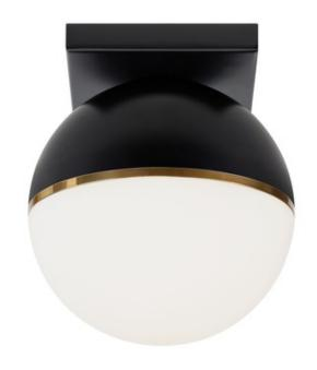
BODY FINISH Matte Black / Bright Brass WATTAGE DIMMER Low Voltage Electronic DIMENSIONS 7"W x 7.8"H INTEGRATED LED MODULE LAMP 1 x LED/120V LED Technical Information LUMINOUS FLUX 641 lumens LUMENS/WATT 45.79 LAMP COLOR 2700K COLOR RENDERING 90 CRI
