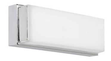
SHADE COLOR N/A **BODY FINISH** Chrome WATTAGE 25W DIMMER Low Voltage Electronic DIMENSIONS 13"W x 4.3"H x 3"D INTEGRATED LED MODULE LAMP 1 x LED/25W/120V LED Technical Information LUMINOUS FLUX 1334 lumens LUMENS/WATT 53.36 LAMP COLOR 2700K COLOR RENDERING 90 CRI
