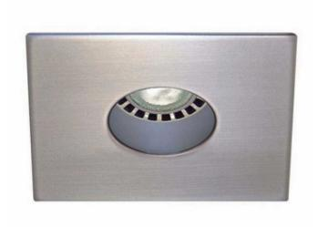
TRIM COLOR N/A BODY FINISH Brushed Nickel/ Anodized Reflector WATTAGE 50W DIMMER Dimmable DIMENSIONS 4.25"W x 2"H x 4.25"D **BULB NOT INCLUDED** LAMP 1 x MR16/GU5.3 (bipin)/50W/12V Halogen 1 x MR16/GU5.3 (bipin)/12V LED 1 x MR16/GU10/120V Halogen 1 x MR16/GU10/120V I ED 1 x PAR16/Medium (E26)/120V LED Technical Information **FUNCTION** Downlight CEILING TYPE Drywall with Trim APERTURE SHAPE Pinhole APERTURE SIZE 1.700" SPEC # CLT51559
