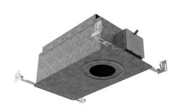
TRIM COLOR N/A BODY FINISH Galvanized Steel WATTAGE 1/1/1/ DIMMER Dimmable DIMENSIONS 19.5"W x 7.06"H x 10"D **BULB NOT INCLUDED** LAMP 1 x LED/14W/120V LED Technical Information LUMINOUS FLUX 1450 lumens LUMENS/WATT 103.57 HOUSING TYPE New construction IC HOUSING HEIGHT APERTURE SHAPE Round
