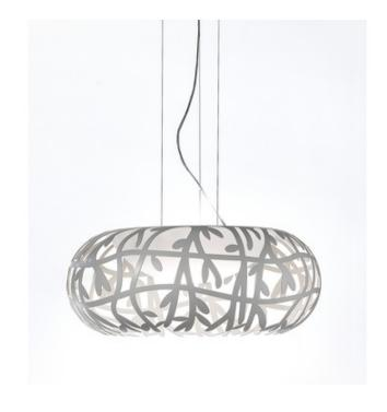
SHADE COLOR Matte White **BODY FINISH** Matte White WATTAGE 17W DIMMER Standard 120V DIMENSIONS 98.42"L x 19.68"W x 14.17"H INTEGRATED LED MODULE LAMP 1 x LED/17W/120V LED Technical Information LUMINOUS FLUX 1800 lumens LUMENS/WATT 105.88 LAMP COLOR 3000K COLOR RENDERING 92 CRI SPEC # SID571857
