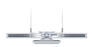
SHADE COLOR N/A **BODY FINISH** White WATTAGE 166\// DIMMER Dimmable DIMENSIONS 28.3"L x 5.1"W x 1.8"H INTEGRATED LED MODULE LAMP 2 x LED/120V LED Technical Information LUMINOUS FLUX 8875 lumens LUMENS/WATT 106.93 LAMP COLOR 3000K COLOR RENDERING 80 CRI SPEC # JDY584605
