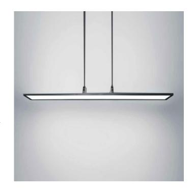
SHADE COLOR White **BODY FINISH** Black WATTAGE 48W DIMMER Low Voltage Electronic DIMENSIONS 46"L x 10"W x 0.88"H INTEGRATED LED MODULE LAMP 1 x LED/48W/120V LED Technical Information LUMINOUS FLUX 3055 lumens LUMENS/WATT 63.65 LAMP COLOR 3000K COLOR RENDERING 90 CRI SPEC # WAC615631
