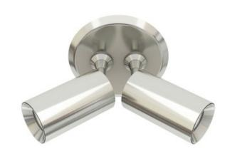
SHADE COLOR **BODY FINISH** Satin Nickel WATTAGE 18W DIMMER Low Voltage Electronic DIMENSIONS 4.6"W x 1.21"H x 3.26"D INTEGRATED LED MODULE LAMP 2 x LED/9W/12V LED Technical Information LUMINOUS FLUX 1034 lumens LUMENS/WATT 114.89 LAMP COLOR 3000K COLOR RENDERING 95 CRI BEAM ANGLE 15°
