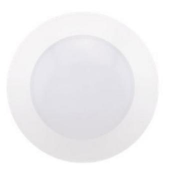
TRIM COLOR N/A BODY FINISH White WATTAGE 11W DIMMER Dimmable DIMENSIONS 7.3"W x 1.3"H INTEGRATED LED MODULE LAMP 1 x LED/11W/120V LED Technical Information LUMINOUS FLUX 680 lumens LUMENS/WATT 61.82 LAMP COLOR 2700K COLOR RENDERING 90 CRI BEAM ANGLE 110° SPEC # GRC621382
