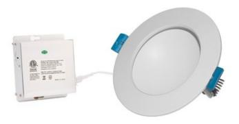
TRIM COLOR N/A **BODY FINISH** Matte White WATTAGE 14\W DIMMER Low Voltage Electronic DIMENSIONS 7.06"W x 2.06"H INTEGRATED LED MODULE LAMP 1 x LED/14W/120V LED Technical Information LUMINOUS FLUX 1080 lumens LUMENS/WATT 77.14 LAMP COLOR 3000K COLOR RENDERING 90 CRI FUNCTION Downlight CEILING TYPE Drywall with Trim HOUSING TYPE Remodel IC HOUSING HEIGHT APERTURE SHAPE Round SPEC # BEA670702
