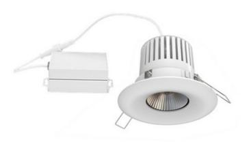
TRIM COLOR N/A **BODY FINISH** Matte White WATTAGE 15W DIMMER Low Voltage Electronic DIMENSIONS 5.25"W x 3"H INTEGRATED LED MODULE LAMP 1 x LED/120V LED Technical Information LUMINOUS FLUX 1500 lumens
