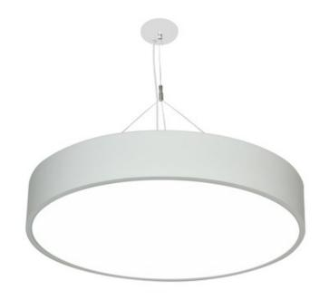
SHADE COLOR N/A **BODY FINISH** Matte White WATTAGE 31W DIMMER 0-10V DIMENSIONS 18"W x 4"H INTEGRATED LED MODULE 1 x LED/120V LED LAMP Technical Information LUMINOUS FLUX 1800 lumens
