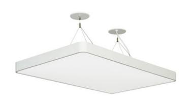
SHADE COLOR N/A BODY FINISH Matte White WATTAGE 92W DIMMER 0-10V DIMENSIONS 122.5"L x 36.75"W x 2.5"H x 15.38"D INTEGRATED LED MODULE LAMP 1 x LED/92W/120V LED Technical Information LUMINOUS FLUX 5500 lumens LUMENS/WATT 59.78 LAMP COLOR 4000K COLOR RENDERING 80 CRI SPEC # ELI751783
