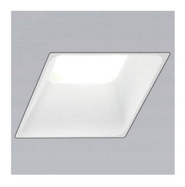
TRIM COLOR N/A **BODY FINISH** White WATTAGE 8 5W DIMMER Low Voltage Electronic DIMENSIONS 2.75"W x 2.56"H x 2.75"D INTEGRATED LED MODULE LAMP 1 x LED/8.5W/120V LED Technical Information LUMINOUS FLUX 700 lumens LUMENS/WATT 82.35 LAMP COLOR 3000K FUNCTION Downlight CELLING TYPE Drywall Trimless/Flush HOUSING TYPE Remodel NON IC HOUSING HEIGHT 5" APERTURE SHAPE Sauare SPEC # ZAN776520
