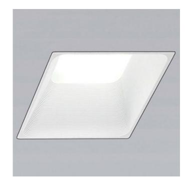
TRIM COLOR N/A **BODY FINISH** White WATTAGE 8 5W DIMMER Low Voltage Electronic DIMENSIONS 2.75"W x 2.56"H x 2.75"D INTEGRATED LED MODULE LAMP 1 x LED/120V LED Technical Information LUMINOUS FLUX 700 lumens LUMENS/WATT 82.35 LAMP COLOR 3000K FUNCTION Downlight CELLING TYPE Drywall Trimless/Flush HOUSING TYPE Remodel NON IC HOUSING HEIGHT 5" APERTURE SHAPE Sauare SPEC # ZAN776520
