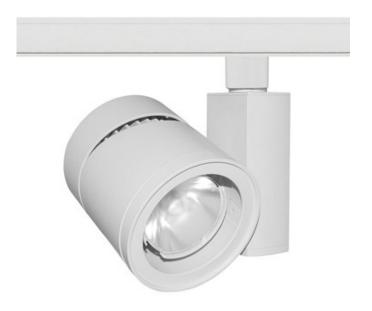
SHADE COLOR N/A **BODY FINISH** White WATTAGE 39\// DIMMER Low Voltage Electronic DIMENSIONS 4.63"W x 6.63"H INTEGRATED LED MODULE LAMP 1 x LED/39W/120V LED Technical Information LUMINOUS FLUX 2446 lumens LUMENS/WATT 62.72 LAMP COLOR 2700K COLOR RENDERING 90 CRI BEAM ANGLE 37° LAMP LIFE 50000 hours FUNCTION Downlight CEILING TYPE Drywall with Trim APERTURE SHAPE Round SPEC # JUN814080
