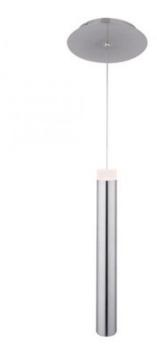
SHADE COLOR White **BODY FINISH** Satin Nickel WATTAGE 7.8W DIMMER Low Voltage Electronic DIMENSIONS 130"L x 1.63"W x 12.38"H INTEGRATED LED MODULE 1 x LED/7.8W/120V LED LAMP Technical Information LUMINOUS FLUX 458 lumens LUMENS/WATT 58.72 LAMP COLOR 3000K COLOR RENDERING 90 CRI
