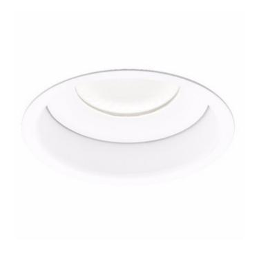
BODY FINISH Matte White/ Matte White Reflector WATTAGE DIMMER Low Voltage Electronic DIMENSIONS 3.5"W x 6.12"H INTEGRATED LED MODULE LAMP 1 x LED/120V LED 1 x LED/120V LED Technical Information LUMINOUS FLUX 1214 lumens LUMENS/WATT 86.71 LAMP COLOR 2700K COLOR RENDERING 90 CRI BEAM ANGLE 40° LAMP LIFE 50000 hours **FUNCTION** Shower/Wet Location CEILING TYPE Drywall with Trim
