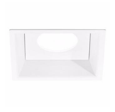
BODY FINISH Matte White/ Matte White Reflector WATTAGE DIMMER Low Voltage Electronic DIMENSIONS 4"W x 6.12"H INTEGRATED LED MODULE LAMP 1 x LED/14W/120V LED 1 x LED/23W/120V LED Technical Information LUMINOUS FLUX 1214 lumens LUMENS/WATT 86.71 LAMP COLOR 2700K COLOR RENDERING 90 CRI BEAM ANGLE 40° LAMP LIFE 50000 hours **FUNCTION** Shower/Wet Location CEILING TYPE Drywall with Trim
