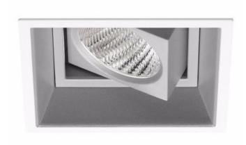
TRIM COLOR Clear **BODY FINISH** Matte White / Natural Anodized Reflector WATTAGE DIMMER Low Voltage Electronic DIMENSIONS 4"W x 6"H INTEGRATED LED MODULE LAMP 1 x LED/14W/120V LED Technical Information LUMINOUS FLUX 1249 lumens LUMENS/WATT 89.21 LAMP COLOR 2700K COLOR RENDERING 90 CRI BEAM ANGLE 15° LAMP LIFE 50000 hours FUNCTION Adjustable Accent CEILING TYPE Drywall with Trim APERTURE SHAPE Square SPEC # CLT835440
