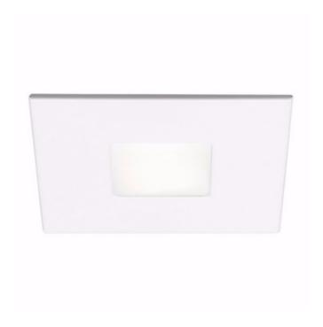
**BODY FINISH** Matte White WATTAGE 10\\\ DIMMER Dimmable DIMENSIONS 4.25"W x 4.38"H INTEGRATED LED MODULE 1 x LED/10W/120V LED LAMP 1 x LED/15W/120V LED Technical Information LUMINOUS FLUX 422 lumens LUMENS/WATT 42.20 LAMP COLOR 2700K COLOR RENDERING 90 CRI BEAM ANGLE 32°
