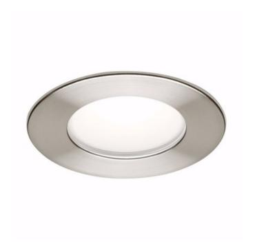
**BODY FINISH** Satin Nickel WATTAGE 15\\\/ DIMMER Dimmable DIMENSIONS 4.87"W x 4.87"H INTEGRATED LED MODULE LAMP 1 x LED/15W/120V LED Technical Information LUMINOUS FLUX 527 lumens LUMENS/WATT 35.13 LAMP COLOR 3000K Warm Dim COLOR RENDERING 90 CRI BEAM ANGLE 32° LAMP LIFE 50000 hours FUNCTION Shower/Wet Location CEILING TYPE Drywall with Trim APERTURE SHAPE Round
