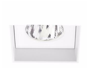
TRIM COLOR Clear **BODY FINISH** Matte White WATTAGE 1/1/1/ DIMMER Low Voltage Electronic DIMENSIONS 3.5"W x 6"H INTEGRATED LED MODULE LAMP 1 x LED/14W/120V LED 1 x LED/23W/120V LED Technical Information LUMINOUS FLUX 1309 lumens LUMENS/WATT 93.50 LAMP COLOR 2700K COLOR RENDERING 90 CRI BEAM ANGLE 15° LAMP LIFE 50000 hours **FUNCTION** Downlight CEILING TYPE Drywall Trimless/Flush APERTURE SHAPE Square SPEC # CLT841302
