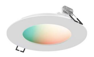
TRIM COLOR N/A **BODY FINISH** White WATTAGE 10\\\ DIMMER Included DIMENSIONS 4.87"W x 1.75"H INTEGRATED LED MODULE LAMP 1 x LED/10W/120V LED Technical Information LUMINOUS FLUX 600 lumens LUMENS/WATT 60.00 LAMP COLOR Tunable White COLOR RENDERING 80 CRI IAMPIIE 50000 hours FUNCTION Downlight CEILING TYPE Drywall with Trim HOUSING TYPE Remodel IC HOUSING HEIGHT SPEC # DLS948461
