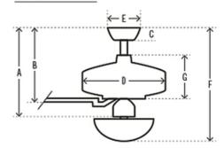
A 19.49 in (Low 18.49 in Angled 52.49 in) B 11.53 in (Low 10.53 in Angled 44.53 in) C 2.77 in D 10.91 in E 6.5 in F 19.49 in (Low 18.49 in Angled 52.49 in)
