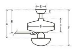
A 12.27 in (Low 11.27 in Angled 45.27 in) B 11.04 in (Low 10.04 in Angled 44.04 in) C 2.75 in D 11.69 in E 6.49 in F 18.17 in (Low 17.17 in Angled 51.17 in) G 4.35 in
