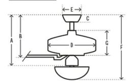
A 19.49 in (Low 18.49 in Angled 52.49 in) B 11.53 in (Low 10.53 in Angled 44.53 in) C 2.77 in D 10.91 in E 6.5 in F 19.49 in (Low 18.49 in Angled 52.49 in)
